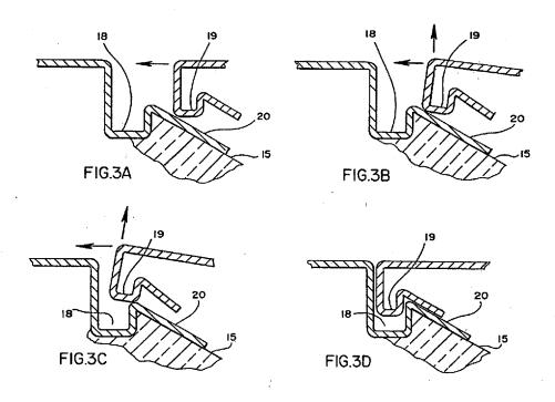
Thus, the operation of the Meyerson element 40 is opposite of the claim 1, which recites: at least one of the one resilient lip and the another resilient lip compresses toward a center of the insert and then springs back out from the center of the insert. This recitation of claim 1 is described, for example, at paragraph 0041 of Applicants' published application (i.e., U.S. Pub. No. 2007/0028547), which states:
